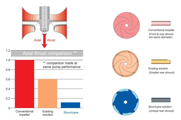
The optimised shape of the Shurricane maintains high efficiencies and very significantly reduces the axial thrust - meaning that any standard IEC motor can be used and bearing life is improved.
