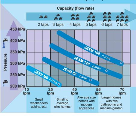
As a simple selection guide, tap symbols are used to represent the flow rate. 1 tap = 10 to 12 lpm
