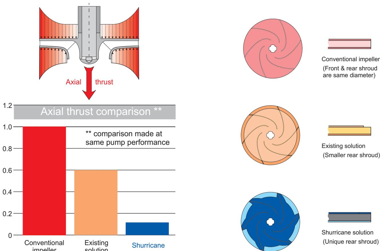
**The optimised shape of the Shurrricane maintains high efficiencies and very significantly reduces the axial thrust - meaning that any standard IEC motor can be used and bearing life is improved.**
